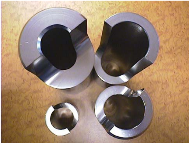
Various sizes of TRES (tube-reduced extrusions) produced at Montreuil-Juigné
