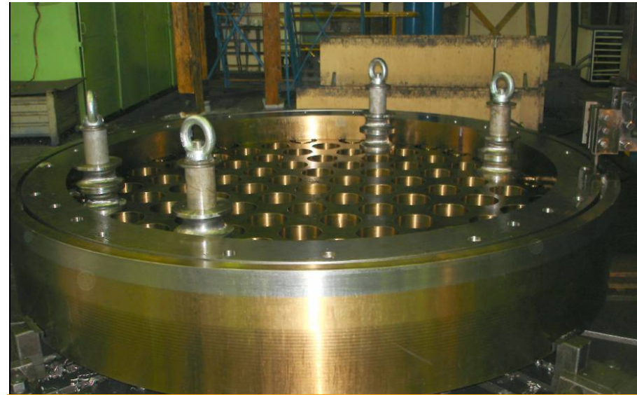
RPV internals: FDD machining
