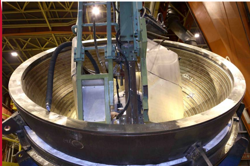
PZR: Buttering of lower head
