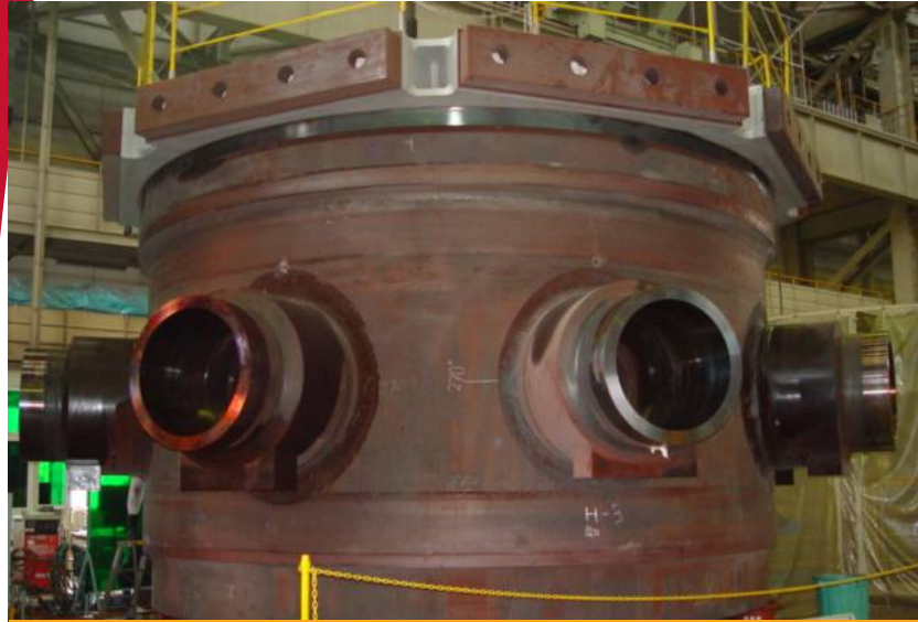
RPV Integrated Shell & Nozzles
