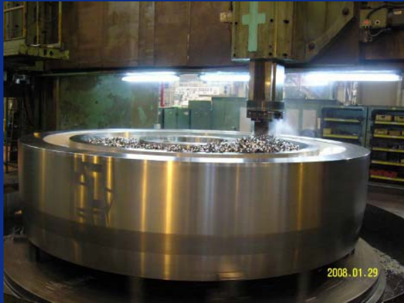
Heavy Component Forgings at Doosan
